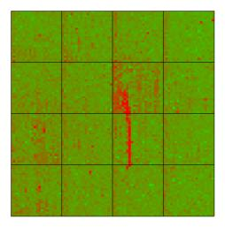
The imageplot function lies the slide on its side, so the first print-tip group is bottom left in this plot. We can see a red streak across the middle two grids of the 3rd row caused by a scratch or dust on the array. Spots which are affected by this artifact will have suspect M-values. The streak also shows up as darker regions in the background plots.
